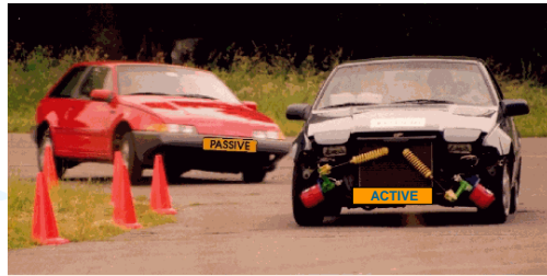
Figure Active suspension systems provide high ride quality or good road holding
