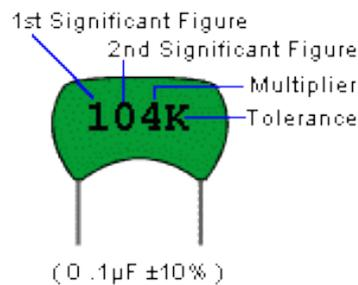
More recently a different type of capacitor coding has come to be in use. In **small types of capacitors such as film or disc form**, instead of the color coding, the capacitance is given as a letter or a number code. The code consists of 2 or 3 numbers and an optional tolerance letter code to identify the tolerance.
