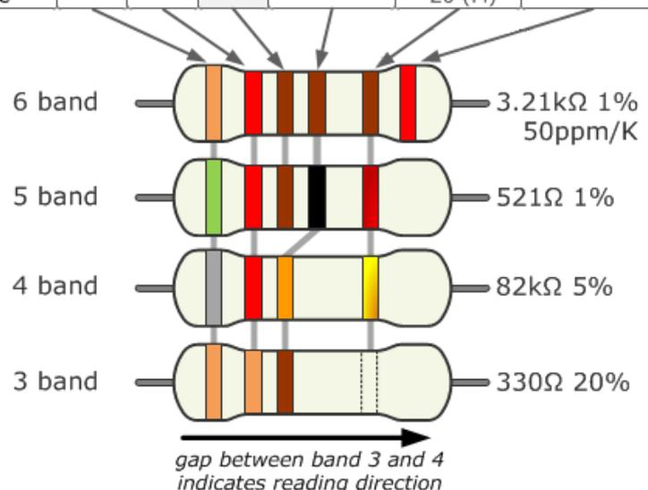
The code shown at the right side is used for the values and tolerances.
